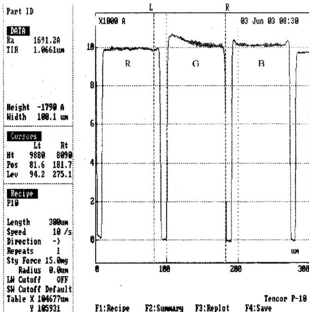
FIGURE 4 — Surface profilometer scan of R, G, B CFs after extended hard-bake.
