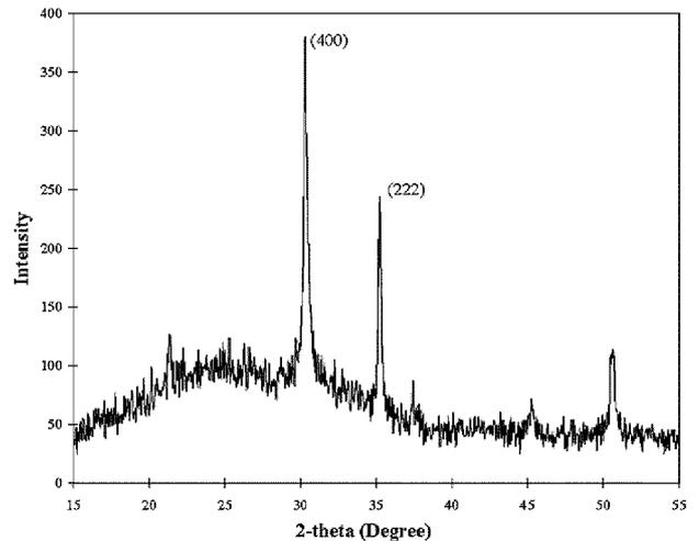
FIGURE 5 — XRD spectrum of room-temperature dc magnetron sputtered ITO on color filters.
