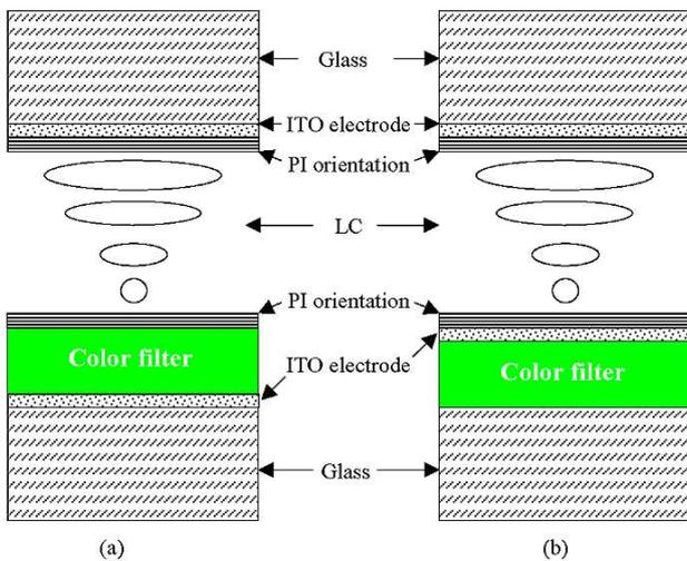
FIGURE 1 — Liquid-crystal cells with rear panels consisting of (a) CF/ITO/glass and (b) ITO/CF/glass.
