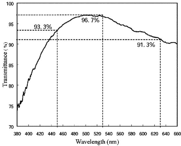
FIGURE 7 — Transmittance spectrum of room-temperature dc magnetron sputtered ITO on glass.
