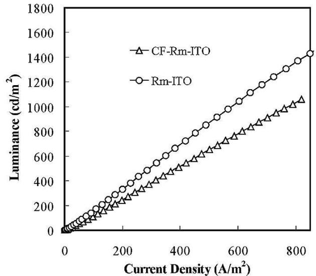
FIGURE 13 — Luminance–current-density characteristics of OLEDs fabricated on room-temperature dc magnetron sputtered ITO on glass and on CF/glass.
