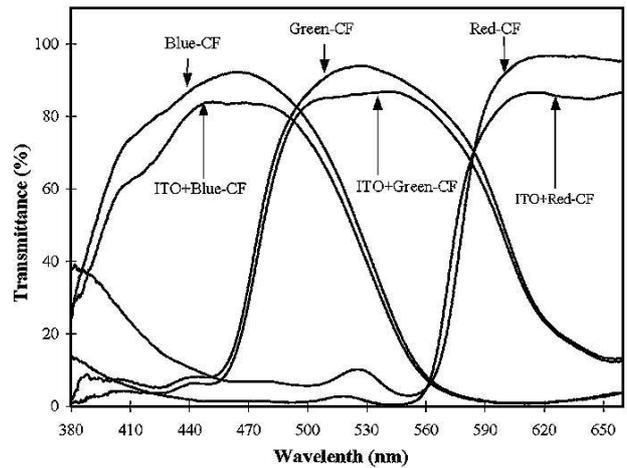
FIGURE 9 — Comparison of the transmittance spectra of red, green, and blue color filters and the same filters covered by ITO.
