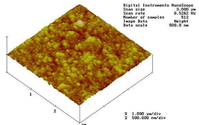
FIGURE 6 — AFM image of room-temperature dc magnetron sputtered ITO on color filters.
