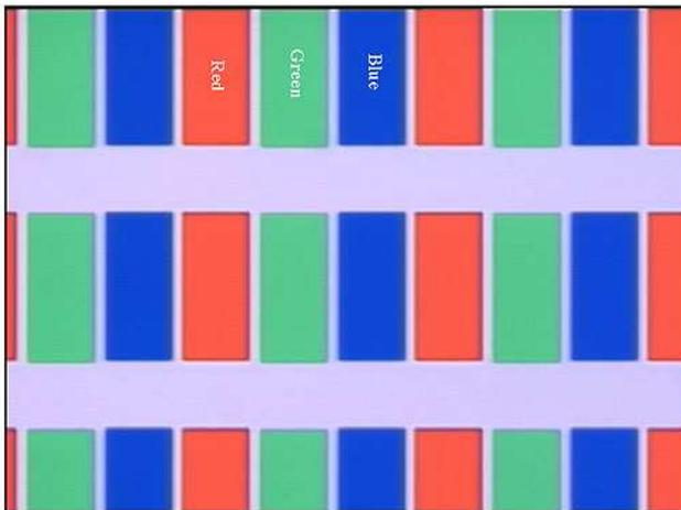
FIGURE 3 — Photograph of micro-fabricated red, green, and blue color-filter array.
