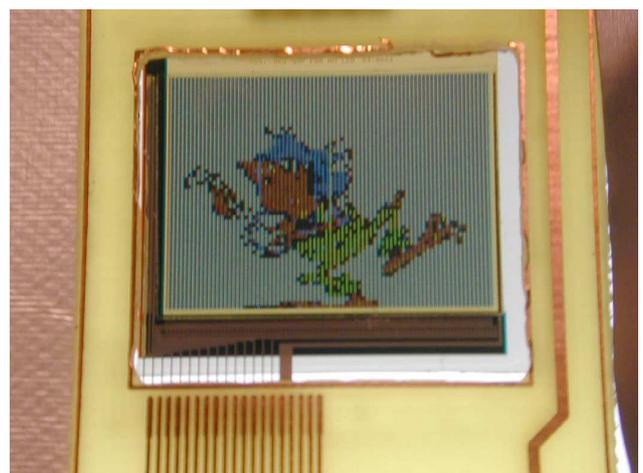
FIGURE 10 — Photograph of an image displayed on MIUC polycrystalline-silicon TFT AMLCD utilizing the technology of room-temperature dc magnetron sputtered ITO on color filters.
