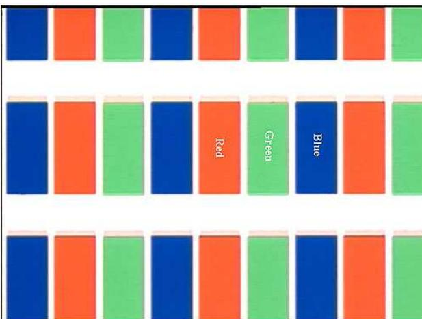
FIGURE 8 — Photograph of a CF array covered by patterned ITO.
