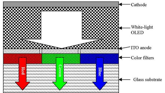
FIGURE 2 — Schematic diagram of a color display based on color filters and white-light-emitting OLED.
