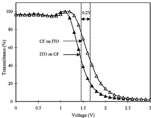
FIGURE 11 — Transmittance–voltage characteristics of LCDs with the two different rear panels.
