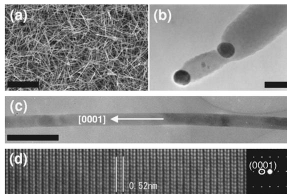
FIG. 1. (a) FE-SEM image shows the as-grown ZnO nanowires (scale bar is 10  $\mu\text{m}$ ). (b) TEM image displays two ZnO nanowires grown from the Au nanoparticle catalysts (scale bar is 15 nm). (c) A ZnO nanowire with diameter of 35 nm illustrates the high aspect ratio geometry (scale bar is 150 nm). (d) Lattice spacing is about 0.52 nm in the HRTEM image and the inset SAED indicates that the growth direction is [0001] along the *c* axis.
