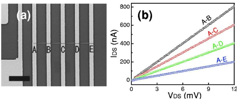
FIG. 3. (Color online) (a) SEM image displays the configuration of a nanowire device contacted with five electrodes, labeled as A-E (scale bar is  $10 \mu\text{m}$ ). (b)  $I_{\text{DS}}-V_{\text{DS}}$  characteristics of a ZnO nanowire measured across subsequent electrode pairs.
