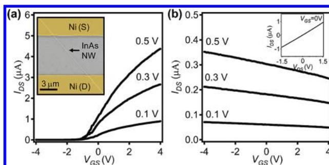
FIGURE 2. The  $I_{\text{DS}}-V_{\text{GS}}$  characteristics of a representative (a) as-grown InAs NW with false-color SEM image of a representative device shown in the inset and (b) blank (i.e., unpatterned) Zn-doped InAs NW with  $I_{\text{DS}}-V_{\text{DS}}$  plot for  $V_{\text{GS}} = 0$  shown in inset. The heavily doped Si substrate is used as the global back gate with a gate dielectric thickness of  $50 \text{ nm SiO}_2$ .
