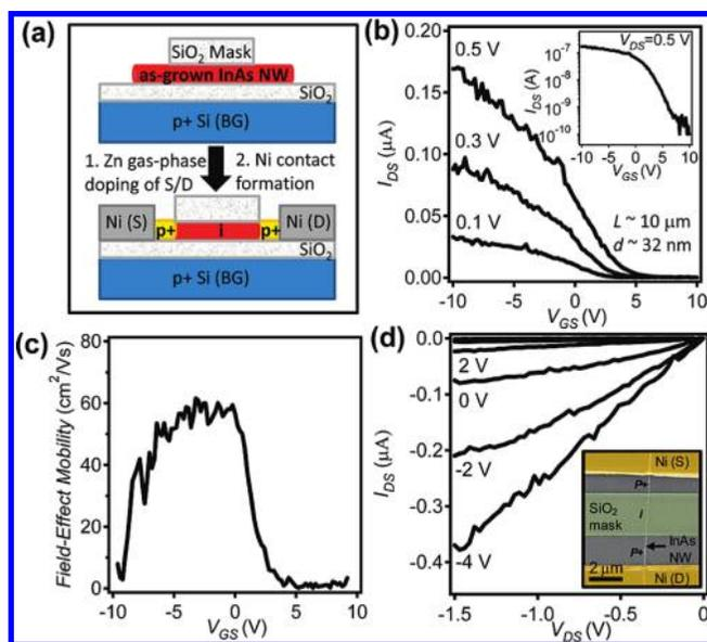
**FIGURE 4.** (a) A schematic of the back-gated InAs NW p-MOSFETs. (b) The  $I_{DS}-V_{GS}$  behavior of a representative p-MOSFET with the log scale plot shown in the inset. (c) Hole field-effect mobility of the device as a function of the back-gate voltage. (d) The output characteristics of the same NW p-MOSFET with false-color SEM image of a representative p-MOSFET shown in inset.
