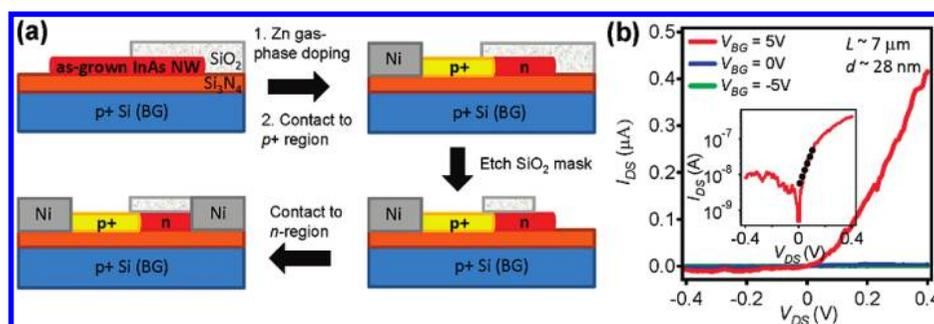
**FIGURE 3.** (a) The process flow for the fabrication of back-gated InAs NW diodes. (b) The  $I$ – $V$  behavior of a representative diode as a function of the back-gate voltage,  $V_{BG}$ . The inset shows the log scale plot for  $V_{BG} = 5$  V and the fit to the ideal diode equation indicated by the dotted line.
