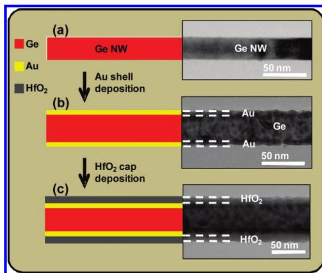
**FIGURE 1.** The fabrication scheme and the corresponding TEM images of the initial Ge/Au core/shell NWs with a 10 nm HfO<sub>2</sub> capping layer. (a) Single-crystalline Ge NWs with diameter  $d = 50$ – $60$  nm are first grown. (b) Au shell with tunable thickness is sputtered on the surface of the NWs. (c) HfO<sub>2</sub> capping layer is deposited on the outer surface by ALD at a sample temperature of 150 °C.
