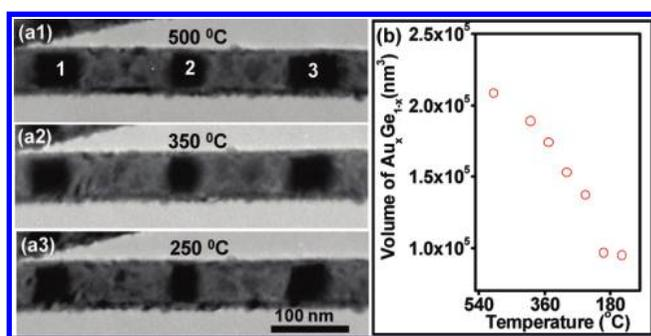
FIGURE 4. In situ TEM analysis for a NW sample with 29–37 atom % Au at (a1) 500 °C, (a2) 350 °C, and (A3) 250 °C. The TEM images correspond to the cool-down step. (b) The total volume of regions 1, 2, and 3 (as labeled in (a1)) as a function of temperature.
