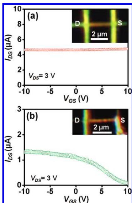
FIGURE 5. Electrical measurements of back-gated devices based on (a) fully alloyed  $\text{Au}_x\text{Ge}_{1-x}$  NW and (b) periodic Au/Ge nanodisk NW, showing metallic and semiconducting behaviors, respectively. The insets show the corresponding dark field optical images of the NW devices.
