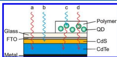
**Figure 3.** Schematic design of a CdTe/CdS solar cell device with a QD-based LDSL deposited on top. (a) Solar radiation is utilized in the active region of the CdTe layer (blue box), apart from high energy UV-blue light (b) which is absorbed by the CdS window layer (yellow box). (c) With the addition of the QD-based LDSL, UV-blue light is absorbed by the QDs and re-emitted in the region of preferential absorption by the solar cell. (d) QDs absorb weakly in the solar cell band's region.
