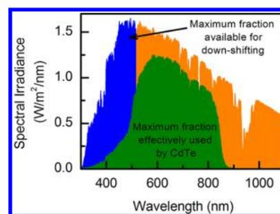
**Figure 1.** Global solar spectrum at air mass 1.5 showing the fraction absorbed by a typical CdTe based photovoltaic device (green) and the spectral region that can be utilized through down-shifting process (highlighted in blue).
