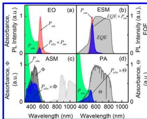
**Figure 2.** Schematic representation of figures of merit used in the model. (a) Emission overlap (EO) integral, (b) emission spectral matching (ESM) integral, (c) absorption spectral matching (ASM) integral, and (d) parasitic absorption (PA) integral.
