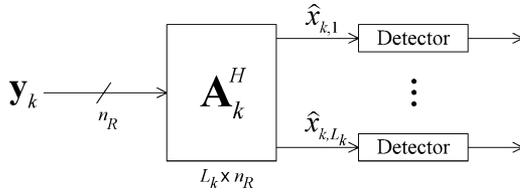
Fig. 3. Independent detection of the substreams.
