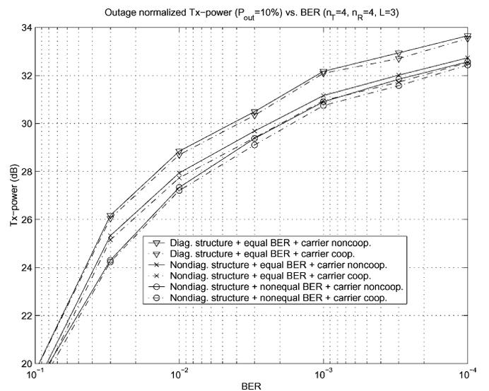
Fig. 8. Outage normalized transmit power versus BER for a multicarrier  $4 \times 4$  MIMO channel with  $L = 3$  (QPSK, 512-QAM, and 512-QAM constellations).
