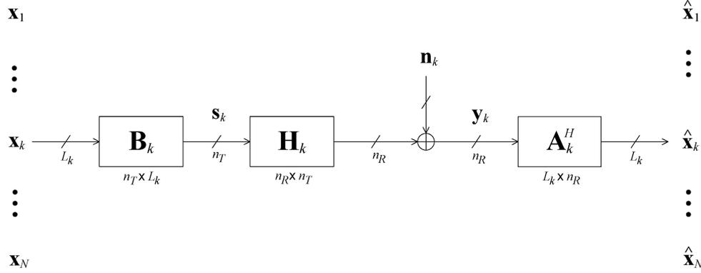
Fig. 1. Block diagram of multiple MIMO channels with linear processing at both the transmitter and the receiver (linear transceivers).
