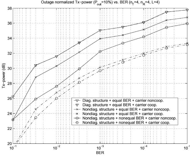
Fig. 9. Outage normalized transmit power versus BER for a multicarrier  $4 \times 4$  MIMO channel with  $L = 4$  (QPSK, 16-QAM, 16-QAM, and 512-QAM constellations).
