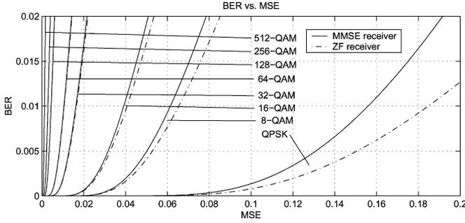
Fig. 4. BER as a function of the MSE for different QAM constellations.
