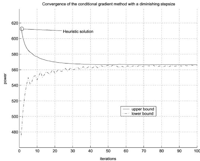
Fig. 6. Convergence of the conditional gradient method for the master problem for a multicarrier  $4 \times 4$  MIMO channel (carrier-cooperative approach) with  $L = 3$  (QPSK, 256-QAM, and 512-QAM constellations).
