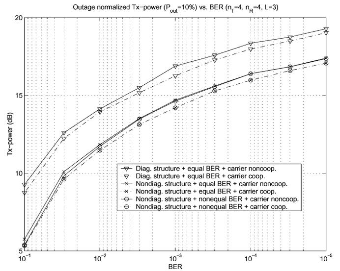
Fig. 7. Outage normalized transmit power versus BER for a multicarrier  $4 \times 4$  MIMO channel with  $L = 3$  (equal QPSK constellations).
